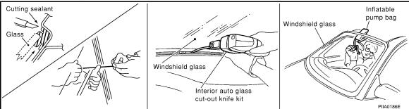
7. Remove the windshield glass, using suction.
