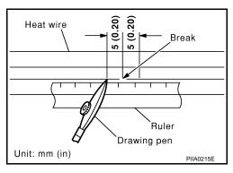
After repair has been completed, check repaired wire for continuity. This check should be conducted 10 minutes after silver composition is deposited.
